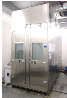
Salt mist testing equipment
