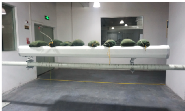
Simulated wind load test
