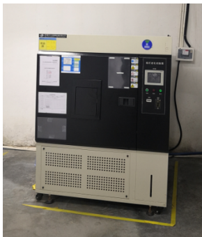
Aging test chamber (Xenon lamp)
